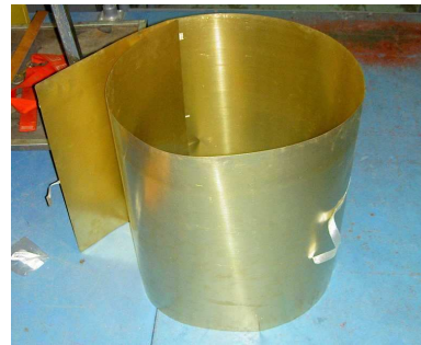
Figure 1. The brass photon converter which was installed in Run3 d -Au experiment (1.7 % radiation length).
