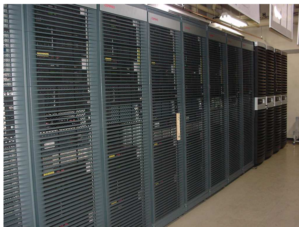
Figure 1. A photograph of the parallel computer system Alphleet-2 comprised of 170 Alpha CPUs. Four racks on the right end were added in 2003 and comprised of 64 CPUs and 96 GB main memory.
