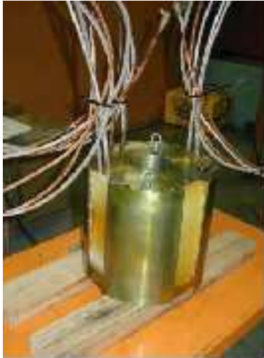
Figure 2. New glaser lens before installation
