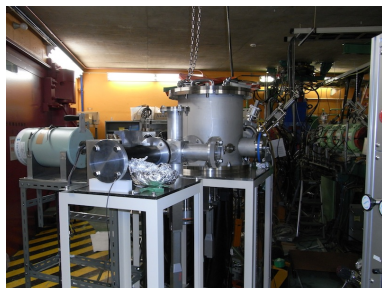
Figure 1. Newly developed scattering chamber located at the E7B course in E7 experimental room
