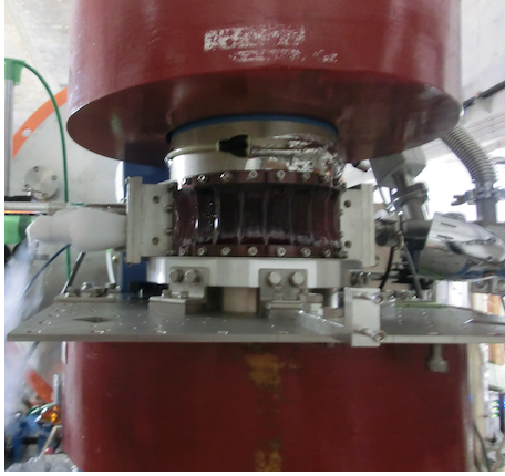
Figure 2. Polarized target chamber installed at the S0 focal plane.
