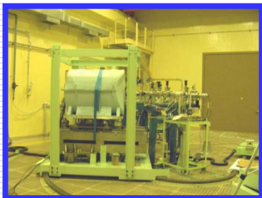
NaI detector Pelletron Facility Neutron beam 100\text{keV} < E_n < 1\text{MeV}
