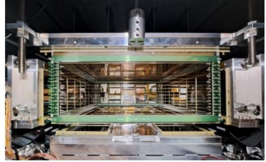
Figure 3: A front view of TexAT\_v2. The field cage is located at the middle of the detector and surrounded by Si and CsI(Tl) detectors.
