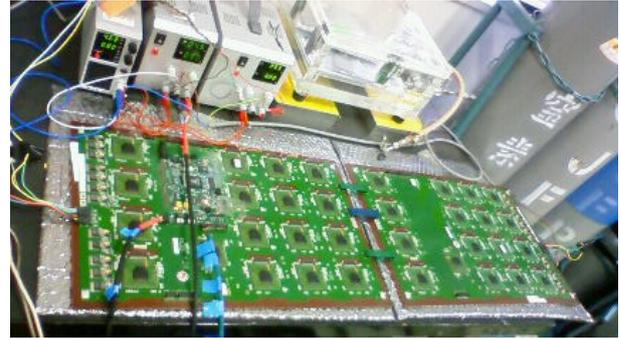
Figure 4. Two ROB, one DCSB and test setup at CNS
