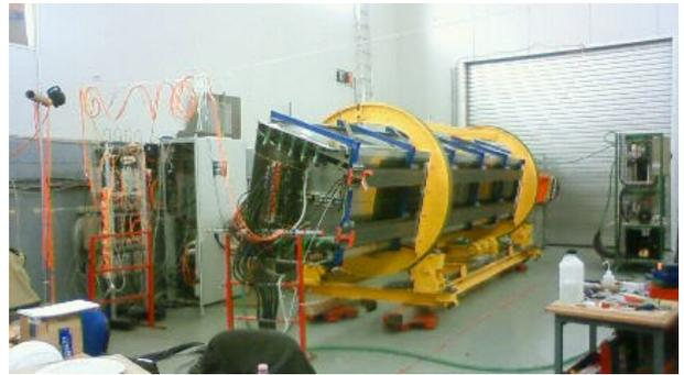
Figure 1. TRD super module in rotator frame at CERN
