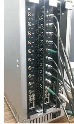
Figure 2. DSP system consisting two 9-ch ADC and our daughter modules (TechnoAP, APU7110-A40) .
