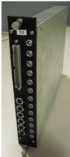
Figure 1. Photo of QTM. 6-inputs, 6-monitor and 1-veto with LEMO connector. The outputs are from 50-pin flat connector. The 6 potentiometer (left bottom) are for the optional input shapers.
