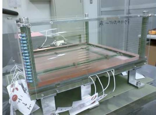
Figure 2. Picture of the field cage of the “beam measurement” type active target.
