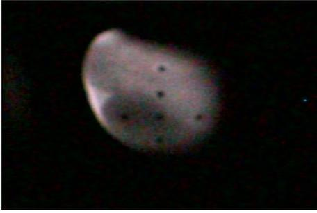
Figure 5. Photograph of irradiated KBr phosphor plate.
