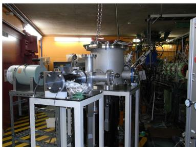
Figure 1. A photo of scattering chamber located at the E7B course in E7 experimental room. There are two target positions for independent experiments of  $\alpha$ -scattering measurement and fusion reaction measurement, respectively.
