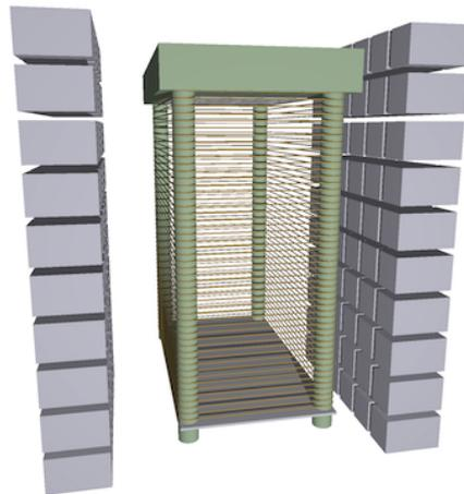
Figure 1. Schematic view of modified active target. One field cage is located along the beam line and two arrays of NaI are located at the both sides of the field cage.
