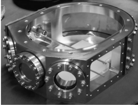
Figure 2. New inner chamber for the polarized target
