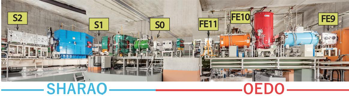
Figure 1. Second half of OEDO beamline and SHARAO spectrometer.
