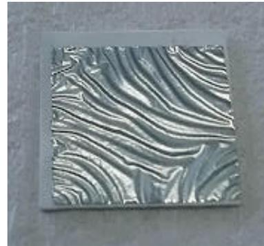
Figure 2. Photograph of target 2, showing the volume expansion after loading with deuterium.
