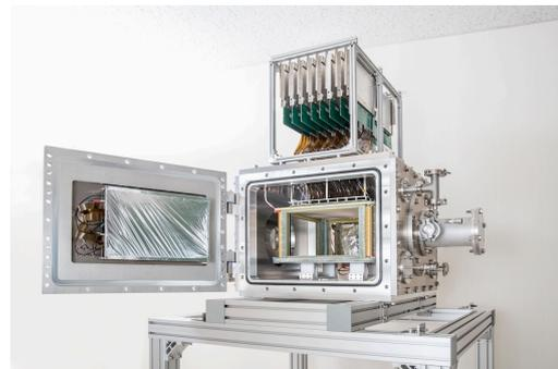
Figure 1. A photograph of CAT-M, which consists of TPC and silicon detectors. The size of active volume is 310×280×200 mm<sup>3</sup>.
