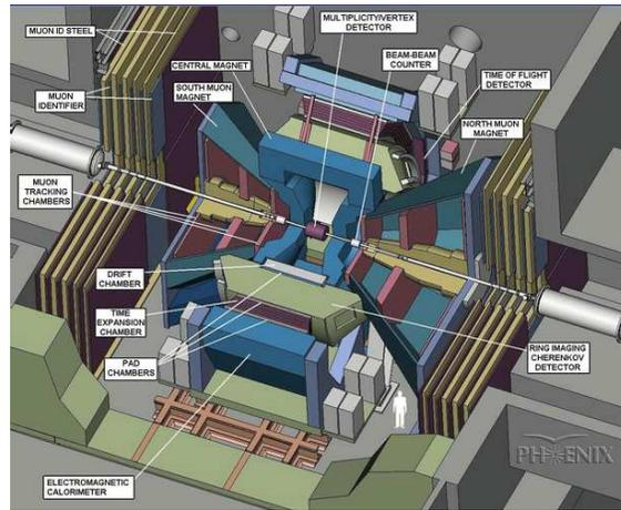
Figure 5.28: A schematic view of the PHENIX experimental setup.
