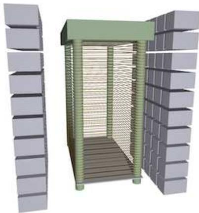
Figure 5.25: Schematic view of the CAT for intermediate-energy high-intensity unstable beam.
