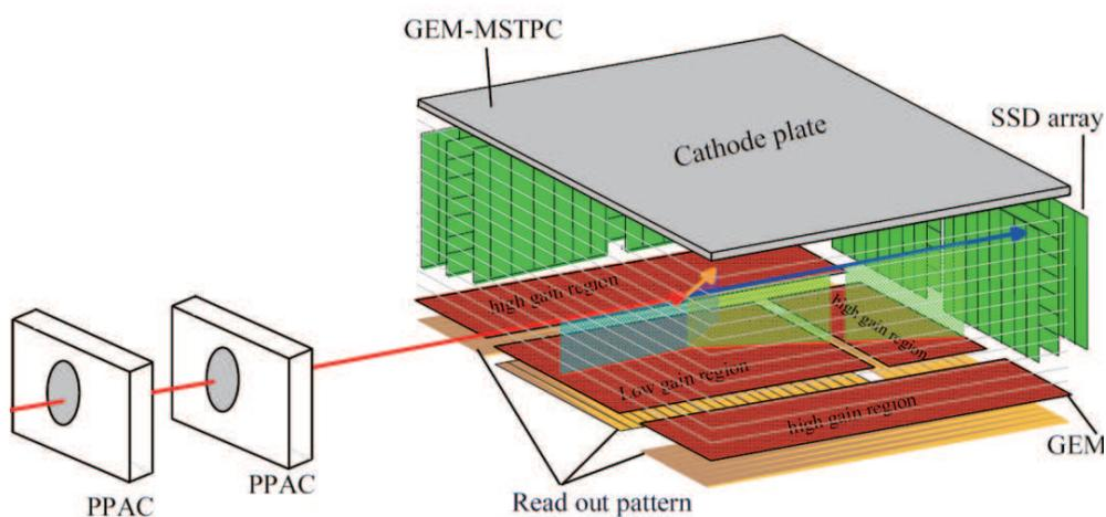
Figure 5.26: Design view of the active target system for nuclear astrophysics studies (GEM-MSTPC).
