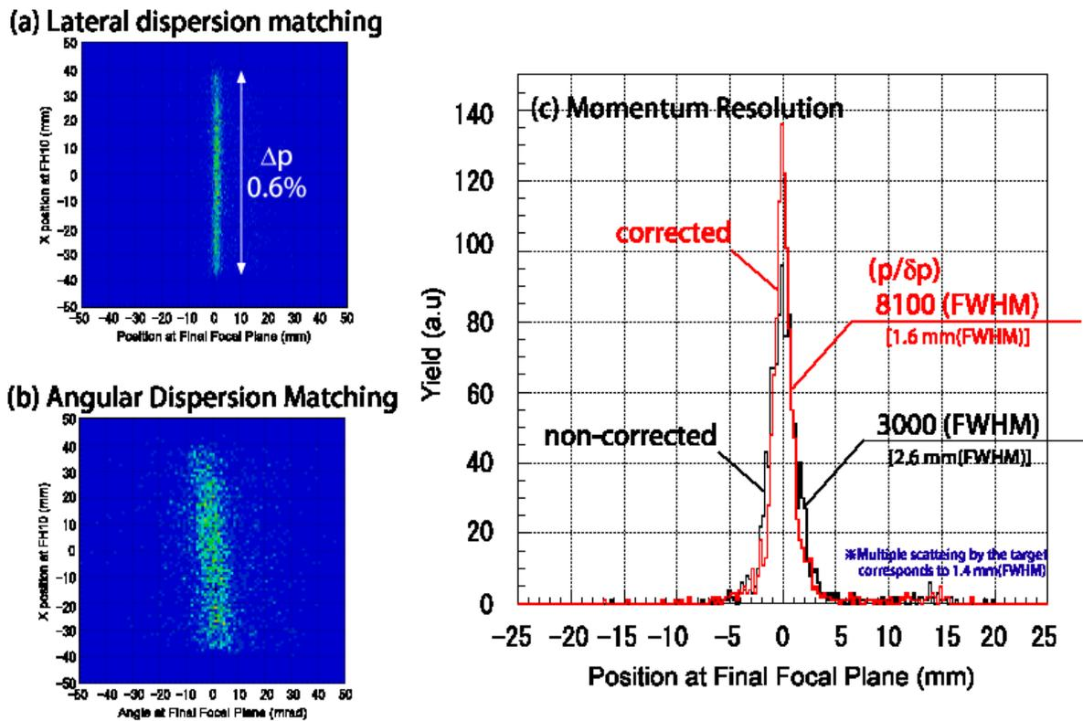
Figure 5.19: Performance of the Dispersion-matching Transport mode. (a) Lateral dispersion matching condition. (b) Angular dispersion matching condition. (c) Momentum resolution.
