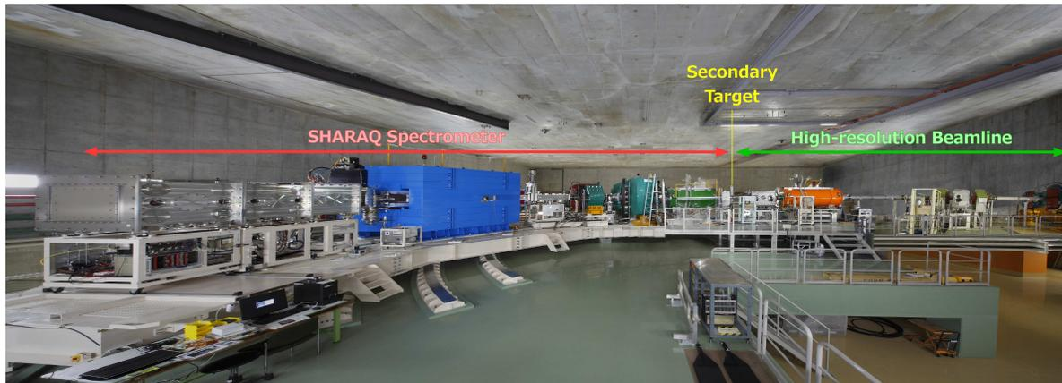
Figure 5.18: Photograph of SHARAQ spectrometer and High-resolution Beamline
