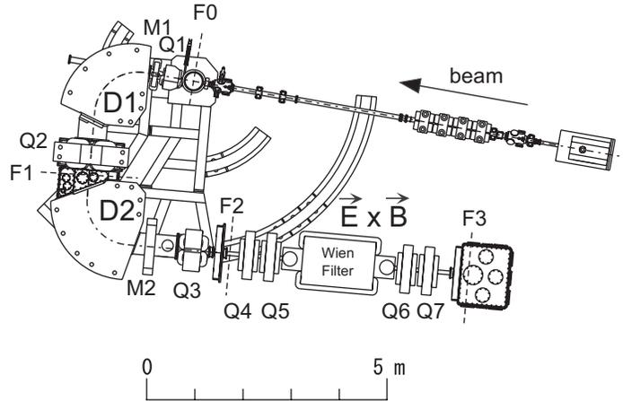
Figure 5.4: Plane view of CRIB. The primary beam is accelerated by the AVF cyclotron of RIKEN. D, Q, and F represent a dipole magnet, a quadrupole magnet, and a focal plane, respectively.
