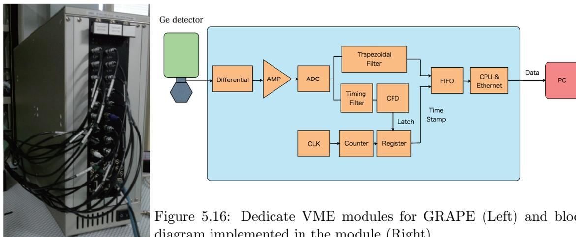
Figure 5.16: Dedicated VME modules for GRAPE (Left) and block diagram implemented in the module (Right).
