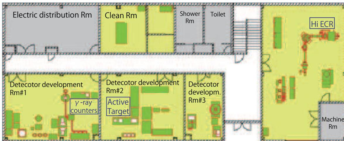
Figure 5.2: The layout of the ground floor of the CNS Research and Development building.
