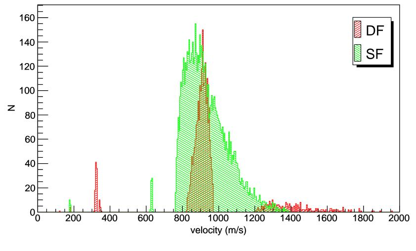
Velocity distribution in MW cavity is wider for SF  $\Rightarrow$  MW resonance is broader
