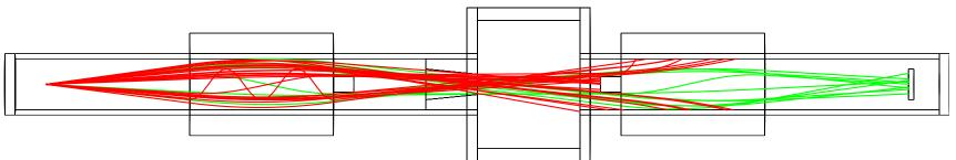
Opening angle: 20°, internal diameter: 10 cm, total length:  $\sim$ 170 cm, pole tip field: 4 T;  $\epsilon \simeq 4 \times 10^{-4}$
