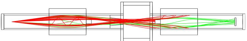
Opening angle: 20°, internal diameter: 10 cm, total length: ~170 cm, pole tip field: 4 T;  $\epsilon \simeq 4 \times 10^{-4}$
