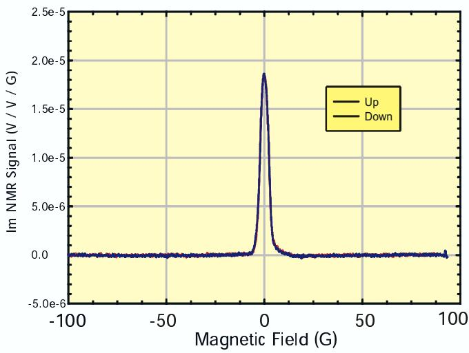
$$\text{NMR Signal} = \frac{2 V_{\text{out}}}{\pi \mu_0 L_0 V_m \mu V_{\text{in}} \eta G_1}$$
