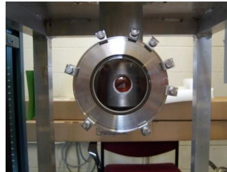
**Liquid Hydrogen target**
